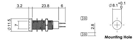
Anode termination indicated by red sleeve. Mounting hole to be clean and burr free.
